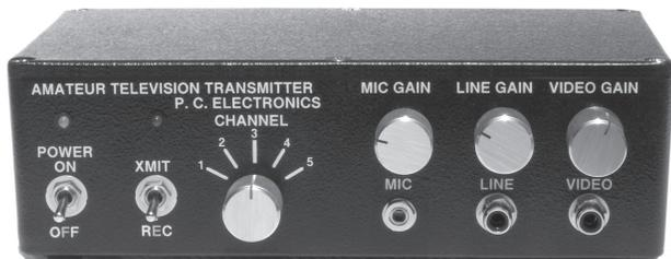
**VIDEO GAIN** control. This sets the white level or depth of modulation of the selected video source. In transmit, the knob should be slowly increased clockwise just to the point of white smearing or blooming as described back to you from a station located at least a quarter mile away. The distant ATV receiving station can describe your picture back to you over 2 meters.
