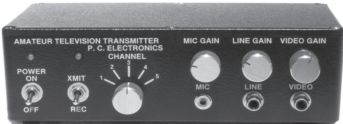
The TX33-.1s transmitter is designed to provide 50-100 milliwatts peak envelope power (sync tip) of video modulated RF in the 33 CM (902-928 MHz) amateur band on any of 5 switch selected frequencies - 910.25, 911.25, 913.25, 919.25 and 923.25 MHz. For higher power, a Downeast Microwave 3340PA linear amplifier can be added.
